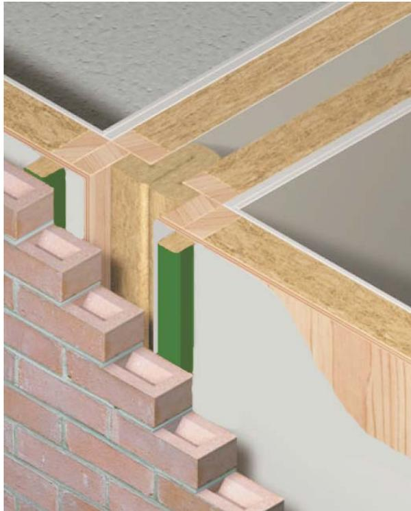
TCB Thermal Cavity Barrier comprises of mineral rock fibre totally enclosed in an oversized polythene sleeve
