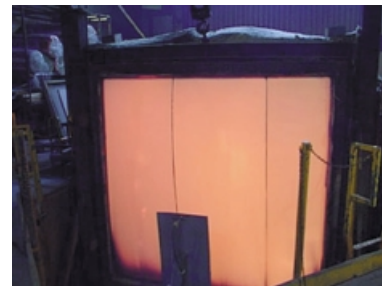
FlameStop60 during fire testing
